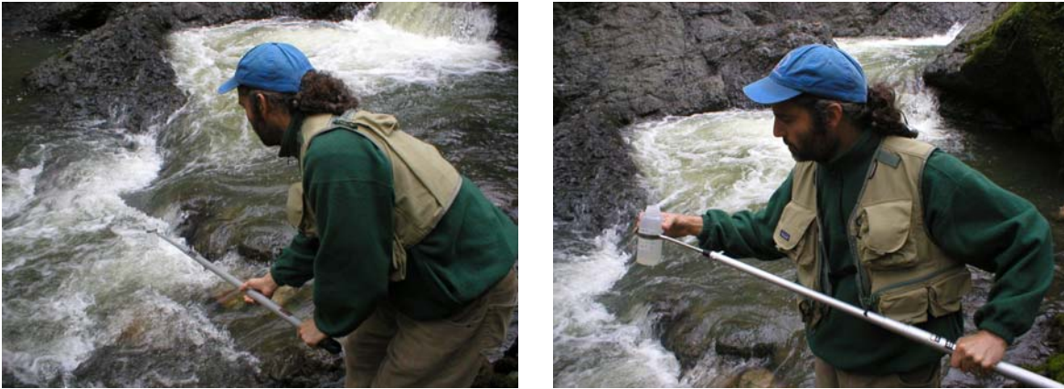
Figure 1. Grab sample collection from the middle of flow using the sampling pole. This photo shows the sample collection into a laboratory sample bottle, but this technique can also be used to collect a grab sample for water quality measurements with field probes if the creek bank or flow conditions make bank access difficult.
